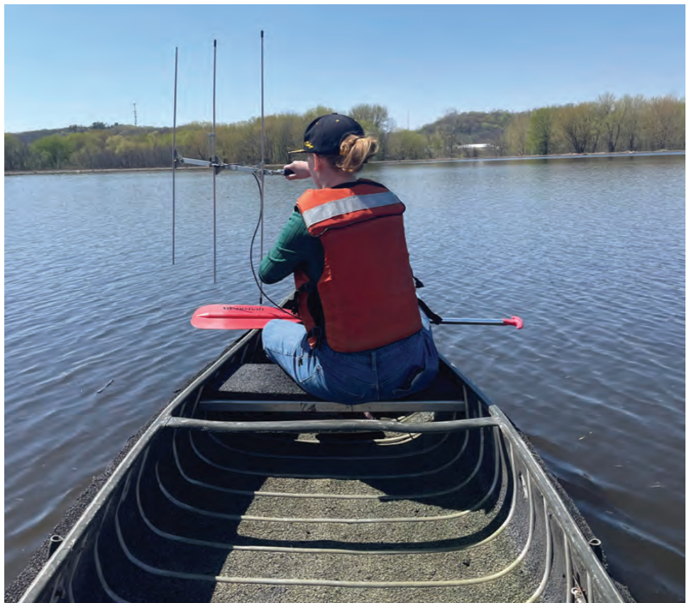
A student uses a radio telemetry receiver and antennae to track Blanding's turtles in a marsh near the Mississippi River.
