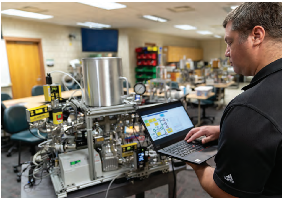
Alumnus Jason Rear demonstrates the automated operation of a vacuum equipment trainer system using his HMI program.
